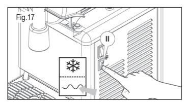
Each bowl is operated by two switches, which must be positioned as follows:
