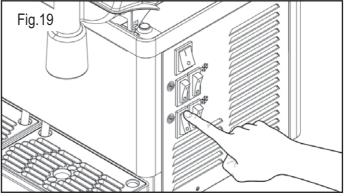
Switch 💥 in position "I" : refrigeration system on.
