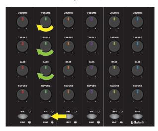
Adjust each channel the same way. Use channel VOLUME knobs to set relative loudness of each channel for overall balance, then adjust MASTER VOLUME knob for overall mix loudness. MASTER VOLUME has a SIGNAL LEVEL METER just to the right; if meter illuminates red, decrease MASTER VOLUME accordingly.
