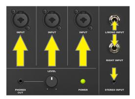
7. POWER UP: Turn on all external equipment connected to Passport first, then turn Passport on. Power LED will illuminate green:
