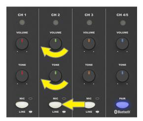
Set up each channel the same way. Use channel VOLUME knobs to adjust relative loudness of each channel until reaching preferred overall balance, then use MASTER VOLUME to adjust overall mix loudness.
